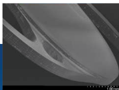
A- Square edge continues at optic haptic junction.
